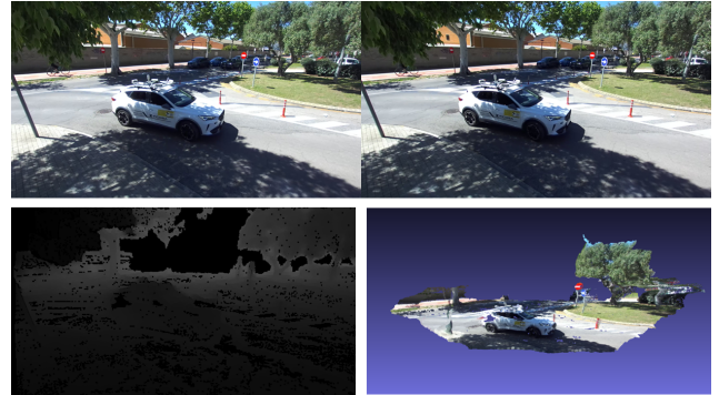
Fig. 4: An example of the frames and point clouds extracted from the static sensor.
